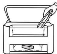
7. If the bubbles cannot be removed, a little alcohol can be poured into the other cup of water, and then place the sample to remove the bubbles.
